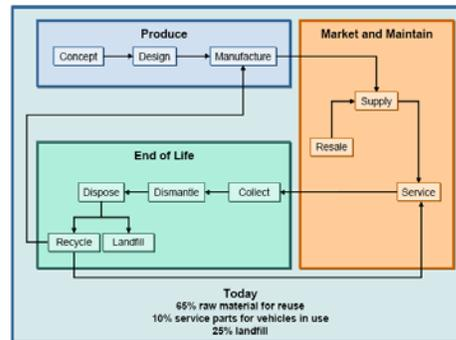
Fig. 4. Design, development, delivery, disposal, and recovery cycle of automotive components, assemblies, and systems
