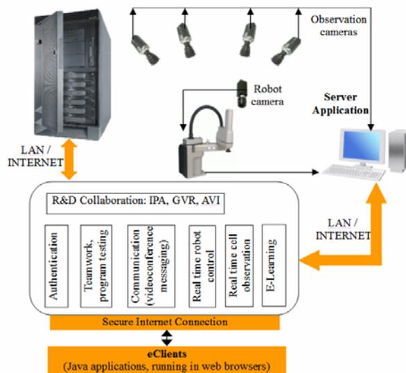
Fig. 1. The structure of the collaboration portal & communication platform
