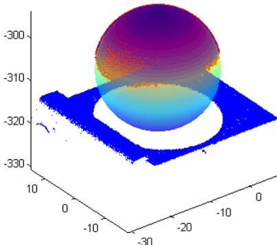
Fig. 3. Sphere identification and fitting from 3D point cloud data.
