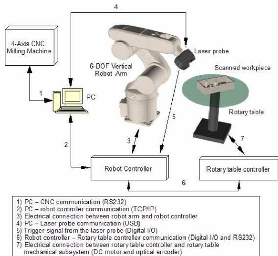
Fig. 1. Overview of the laser scanning system
