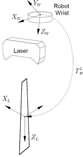
Fig. 2. Tool transformation for the laser probe.
