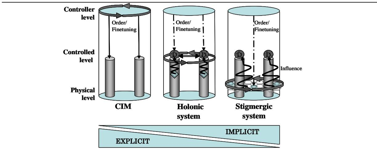
Fig. 4. Control architectures comparison using the open control paradigm
