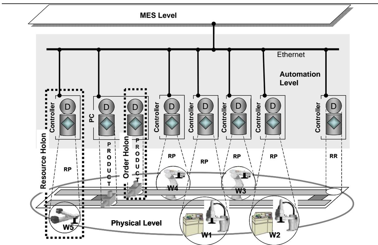
Fig. 6. Holons in the job shop-type FMS and their localization according to the open-control model
