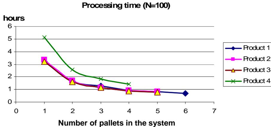
Fig. 8. Execution time as a function of the number of pallets for 100 products of the same type
