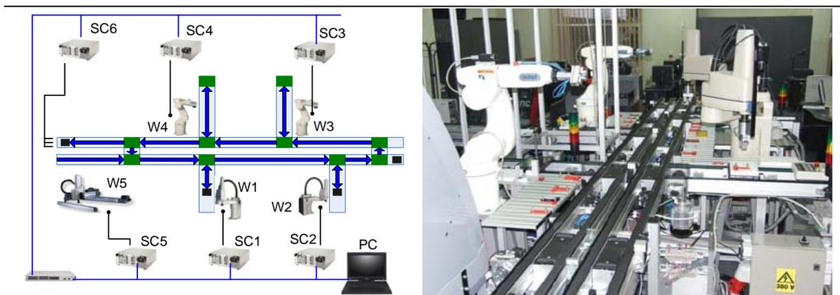
Fig. 5. The production cell with networked robotized workstations: layout (left) and realization (right)
